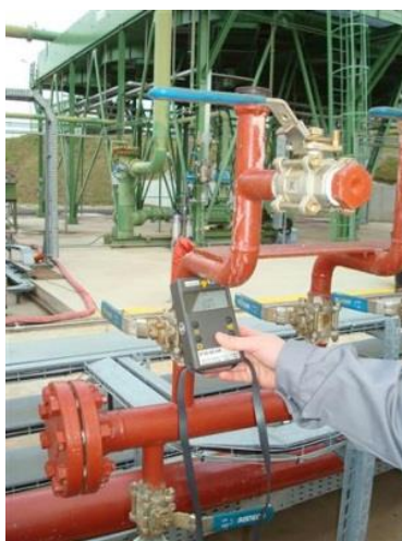
Figure 9: Dose rate measurement performed with a radiometer on a pipe at the Soultz-sous-Forêts power plant (Cuenot et al., 2013).
